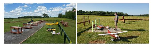
There are two starting pads and one blast deflector for turbine aircraft. Position the model to direct the exhaust over the concrete pad and through the blast deflector.
