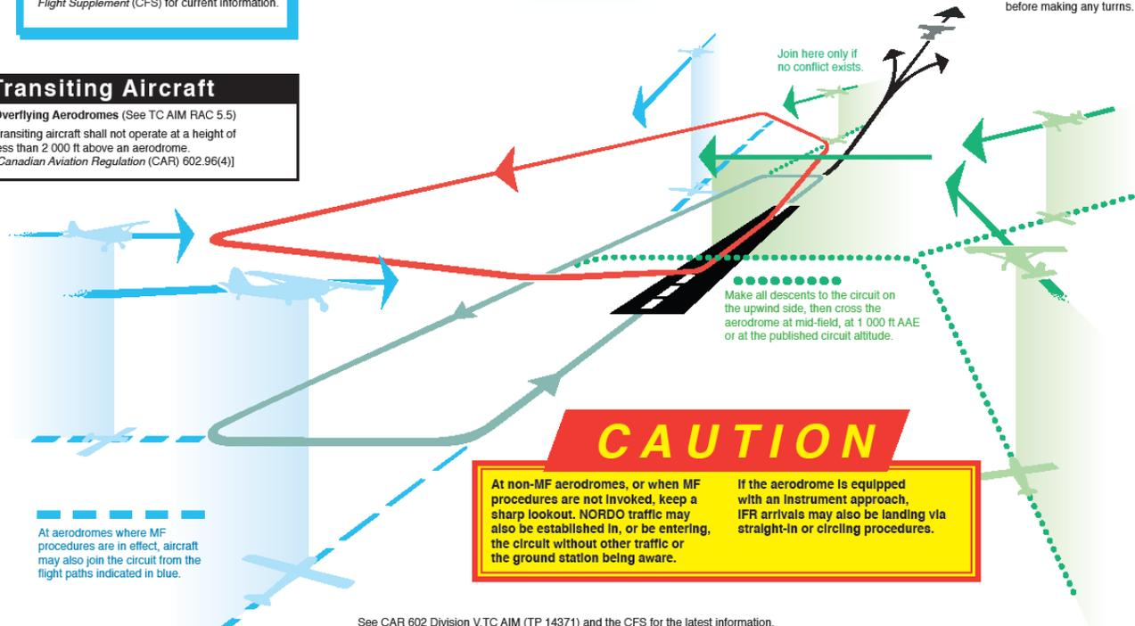
At aerodromes where MF procedures are in effect, aircraft may also join the circuit from the flight paths indicated in blue.
