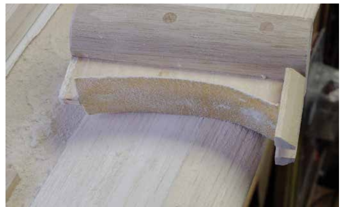
I made up a profile sander too. This was more useful for checking the profile than for actual shaping.
