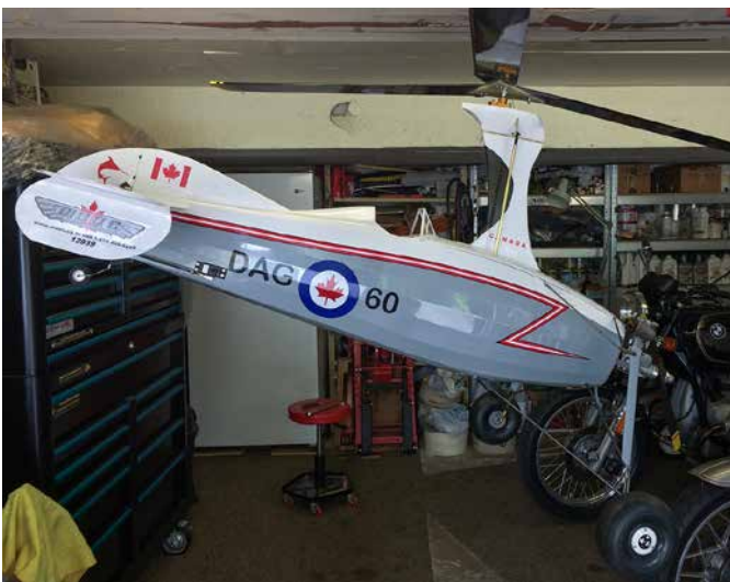
The hang angle is measured under the flat bottom stabilizer. According to the plans, it should be between 14 to 18 degrees as a starting point.
