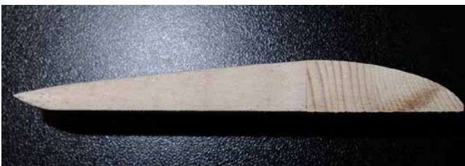
Cross section of my DAG 60 rotor blade.
