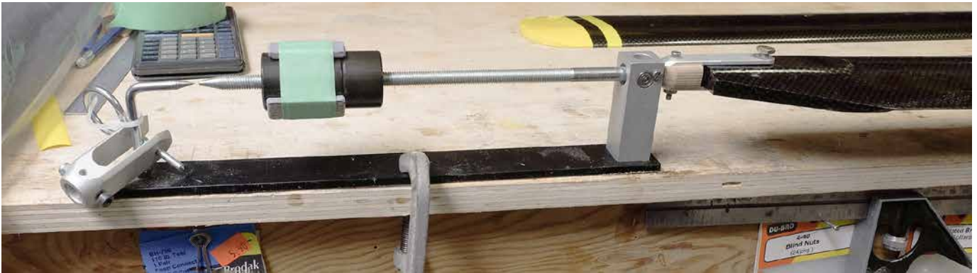
I covered each blade with iron-on film and ensured each weighed the same after covering. This seems laborious but is necessary for a smooth turning rotor.
