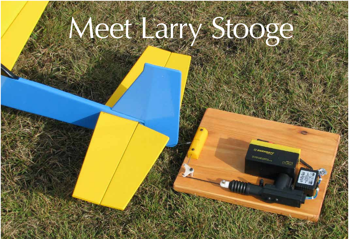
Your Remote Release Airplane Launcher, Larry for short, in use with a Sig Twister powered by an OS 35FP.
