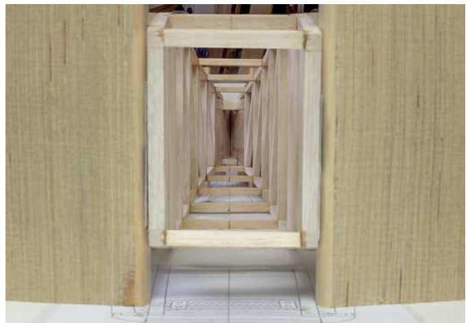
Fuselage in my jig to keep it straight
