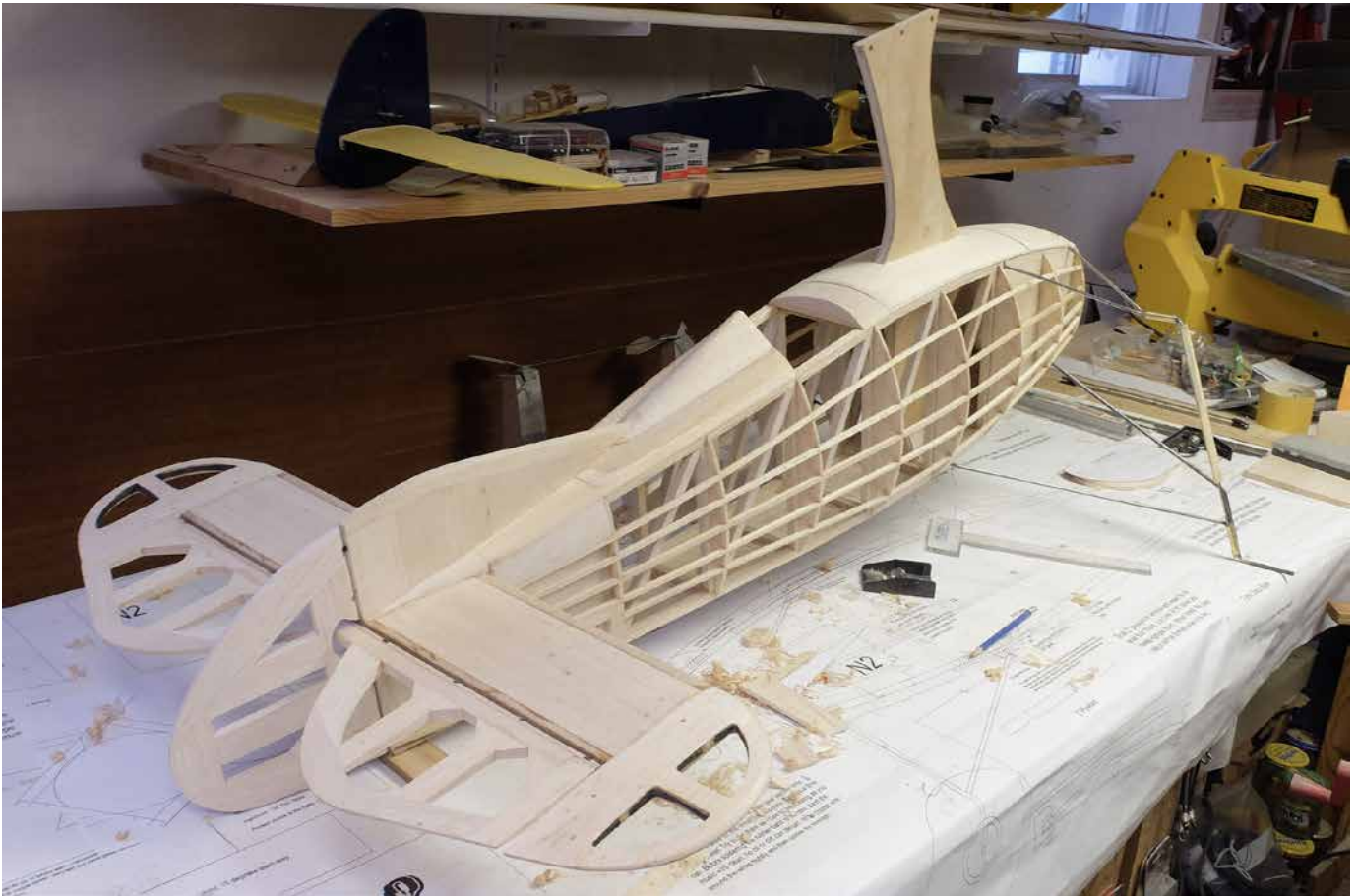
My mast has a 1/4" hard balsa core, 5 oz glass cloth and 1/8" ply epoxied on each side. Very strong.
