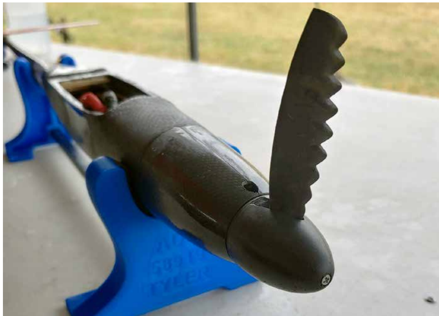
One of the Australian team members used this wild-looking reverse rotation 'shark-tooth' prop to good effect!
