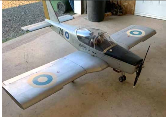
Alf's giant scale Valmet. A training aircraft commissioned by the Finnish Air force in the 1980's. Alf modified the leading edge on the wings for extra lift and installed pneumatic retractable landing gear. This is truly a work of art.
