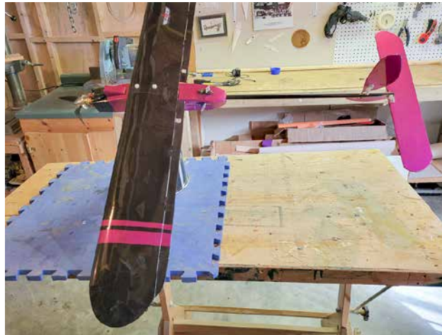
A rescued carbon fiber wing spar from the garbage bin inspired this boom fuselage with all moving pull tail. Looks a bit strange but it flies quite well.
