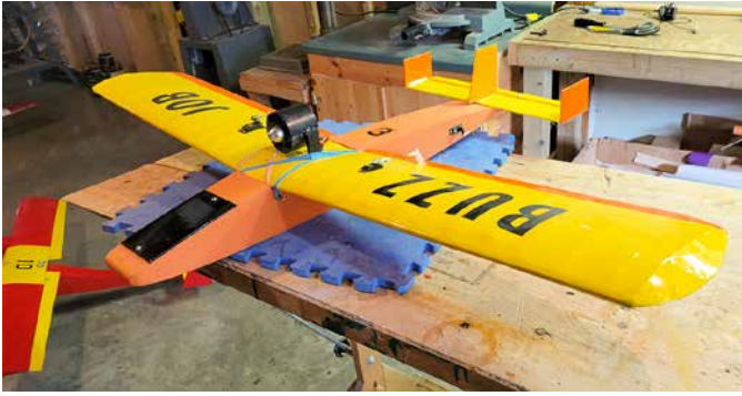
A ducted fan rescued for a Vampire foamy powers this one. Lifting fuselage is because it needs all of the lift it can get. No worries about going supersonic.
