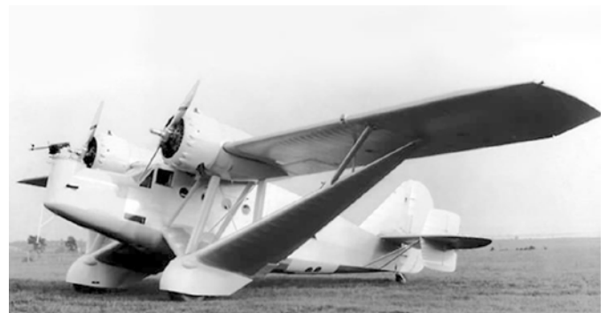
What is not to like: twin engine bomber, nose turret & gull shaped underwing? Bellanca 77-140 Bomber, Introduced early 1930's 1000aircraftphotos.com, David Horne Collection
