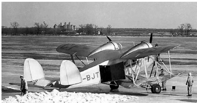
Nugly to the bone, twin engine with inverted gull winglet below main wing. Fleet 50K Freighter, introduced 1938 PHOTO: 1000aircraftphotos.com, Dan Shumaker Collection
