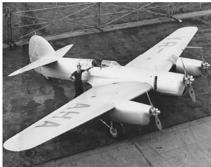
A tri-motor on a fairly small plane. Bellanca 28-92 racer, introduced 1937
