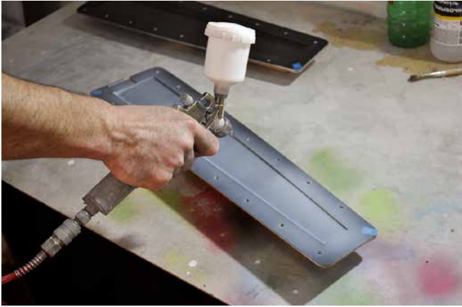
Application of mold release.
