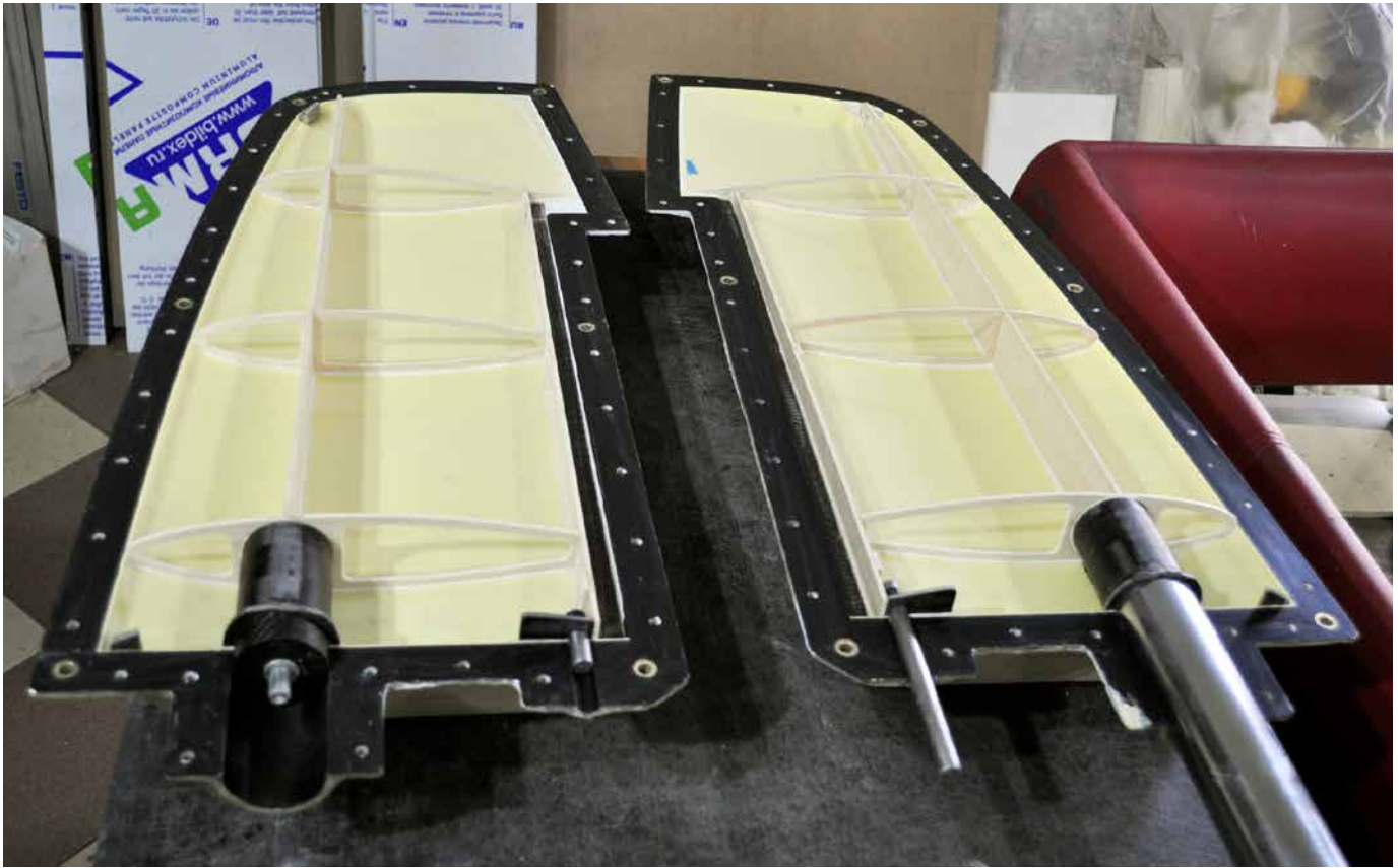
Wing skins with ribs in place.
