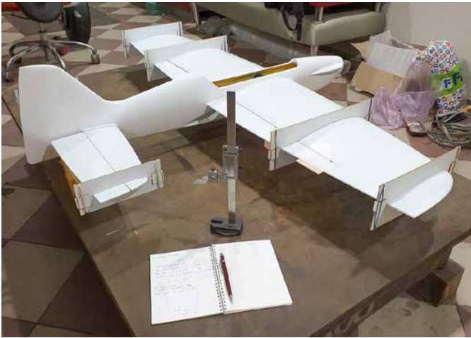
Alignment jig for flying surfaces.
