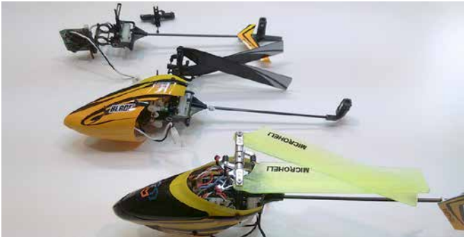
Buying another similar used model, even if not flying, can be a great place to find parts by "frankensteining" them to serve your flyer. These can generally be had for pennies on the dollar when available.
