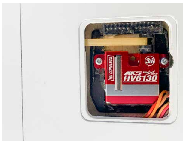
Twister uses an Integrated Drive System (IDS) in wing to eliminate the drag of external control horns.
