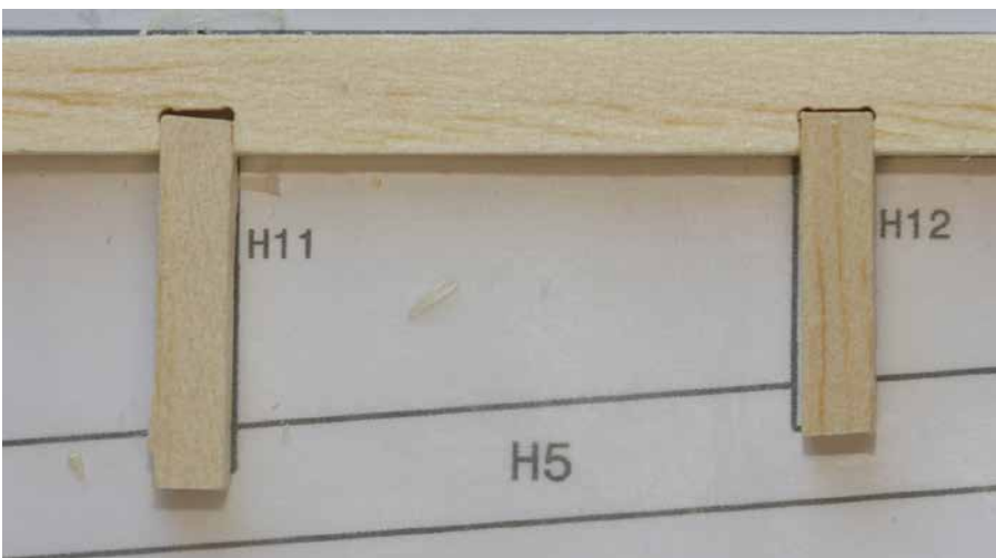
Every piece of the kit is CNC cut, so when I dry assembled H11 and saw thus poor fit... I knew I had done something wrong... I quickly realized I had it the wrong way around. Some of the joints in my Drifter II may have looked like this.
