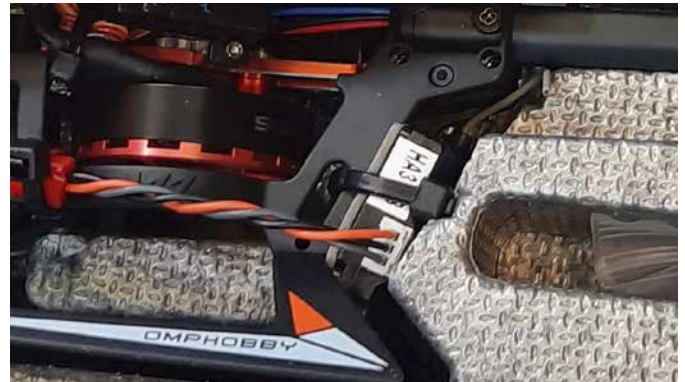
After shaving a little foam off to fit the DSMX receiver addition.
