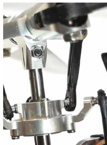
Bolt recess allows for Jesus bolt to be secured without a wrench or pliers.
