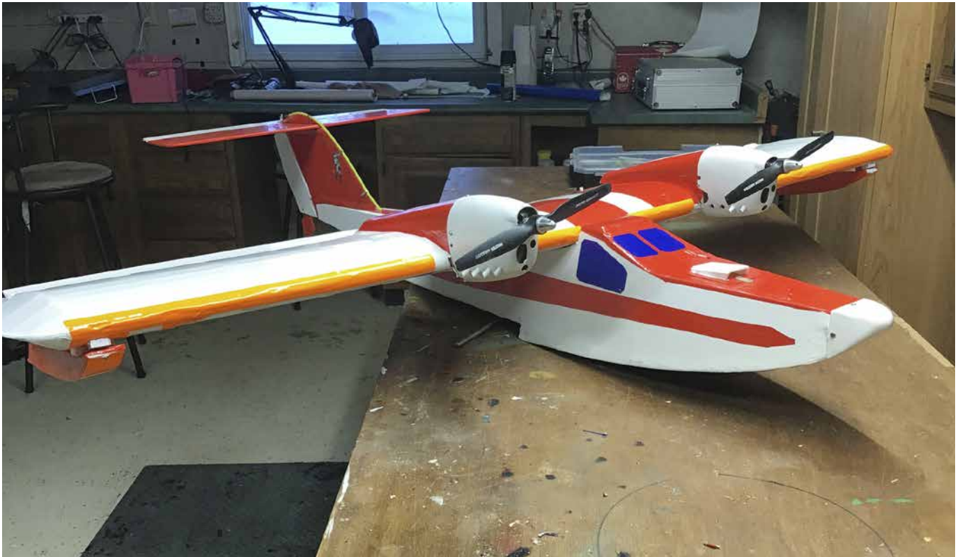
Ace Seamaster rebuilt by Bill Fry ready for the 2021 flying season on Parkhill Lake, 58 inch span, 7 pounds ready to fly,
