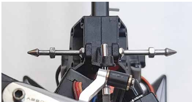
Aggressive ridges on the aluminum canopy posts make quick work of the stock grommets.
