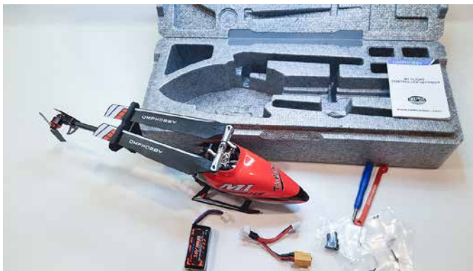
Kit contains, Manual, 1 battery, charge lead, various spares a wrench and a straight driver
