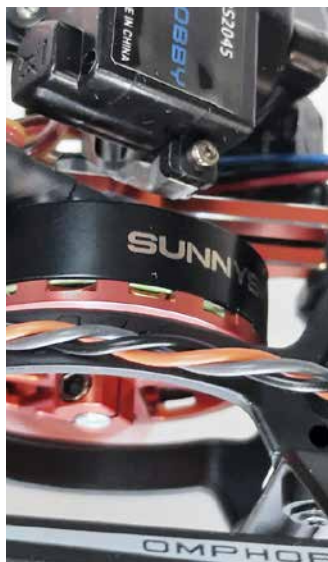
3mm main shaft runs straight through everything including the motor and is secured with a through bolt underneath it all. No gears, pinions or belts, just power with zero play.
