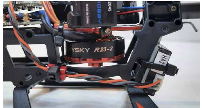
DSMX was installed at the back of the mainframe with foam gyro tape and a zip tie.
