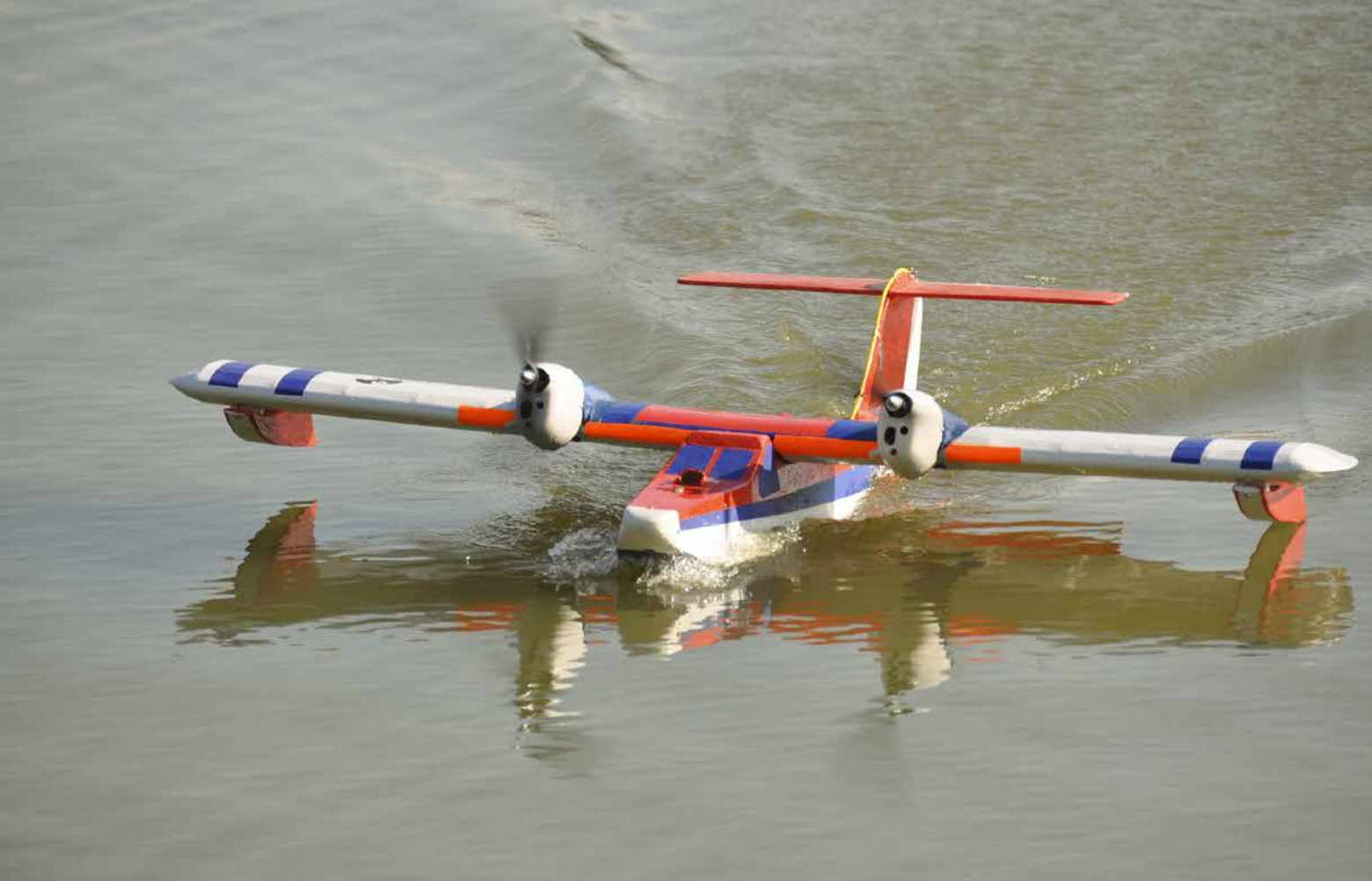
Ace Seamaster, converted to twin electric 25's by Bill Fry, 58 inch span, 7 pounds ready to fly at the Parkhill lake flying site.
