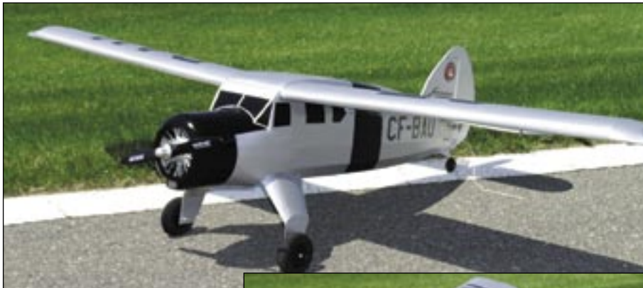
Ottawa's Rob Zinck built this 63" wingspan Noorduyn Norseman from a Unionville Hobbies kit but heavily modified it. It is powered by an Aveox 1406/3Y with a 3.7:1 planetary gear and it runs on 5 Emoli lithium cells (made in Canada) through a CC Phoenix 45HV ESC. All-up weight is 97 oz.
