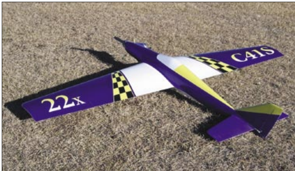
Randy Smith's new Quarter Midget 40 pylon racer, Proud Bird, manufactured by Terence Palaschuk from Fly Fast Composites in Regina, SK. Wing span – 56", Weight – 4 lbs. / Le nouveau Quarter Midget 40 de Randy Smith, le Proud Bird, que fabrique Terence Palaschuk (Fly Fast Composites) à Regina. Envergure : 56 pouces et poids : quatre livres.
