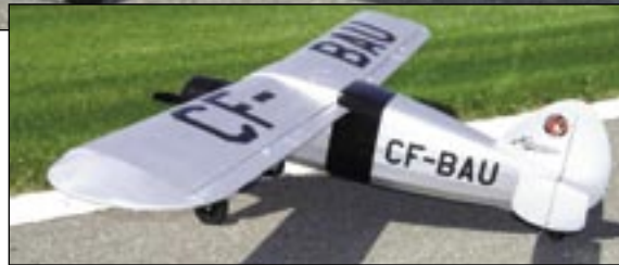
Ottawa's Rob Zinck built this 63" wingspan Noorduyn Norseman from a Unionville Hobbies kit but heavily modified it. It is powered by an Aveox 1406/3Y with a 3.7:1 planetary gear and it runs on 5 Emoli lithium cells (made in Canada) through a CC Phoenix 45HV ESC. All-up weight is 97 oz.
