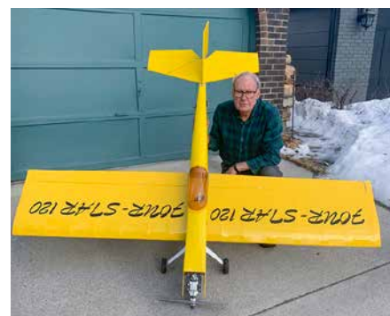
Four Star 120, built by Bob Smyth #2007 of the Chinook Winds R/C Club (Calgary). 80-inch wingspan, 10 pounds, powered by a DLE 20. / Bob Smyth (MAAC 2007) du Chinook Winds Club (Calgary) a construit ce Four Star 120 (du fabricant SIG). Envergure de 80 pouces, poids de 10 livres, mû par un DLE 20. PHOTO: Bob Smyth
