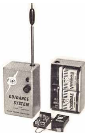
Single channel transmitter with receiver, circa mid 1960 - similar to the author's.
