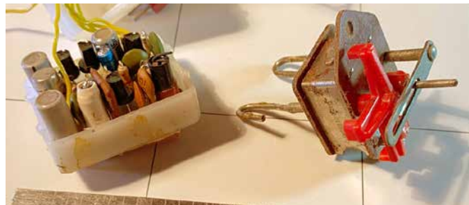
Actual receiver and escapement used in the author's Deacon model.
