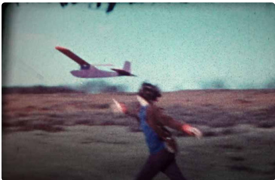
The Deacon is launched - controlled by single channel (rudder only).
