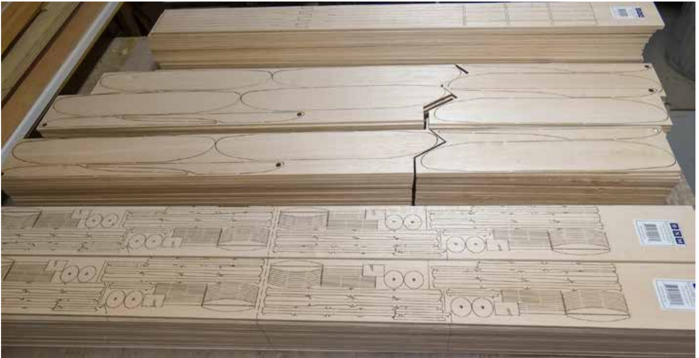
300 Minnow kits and 200 Sparrow kits ready for separation and part assembly.
