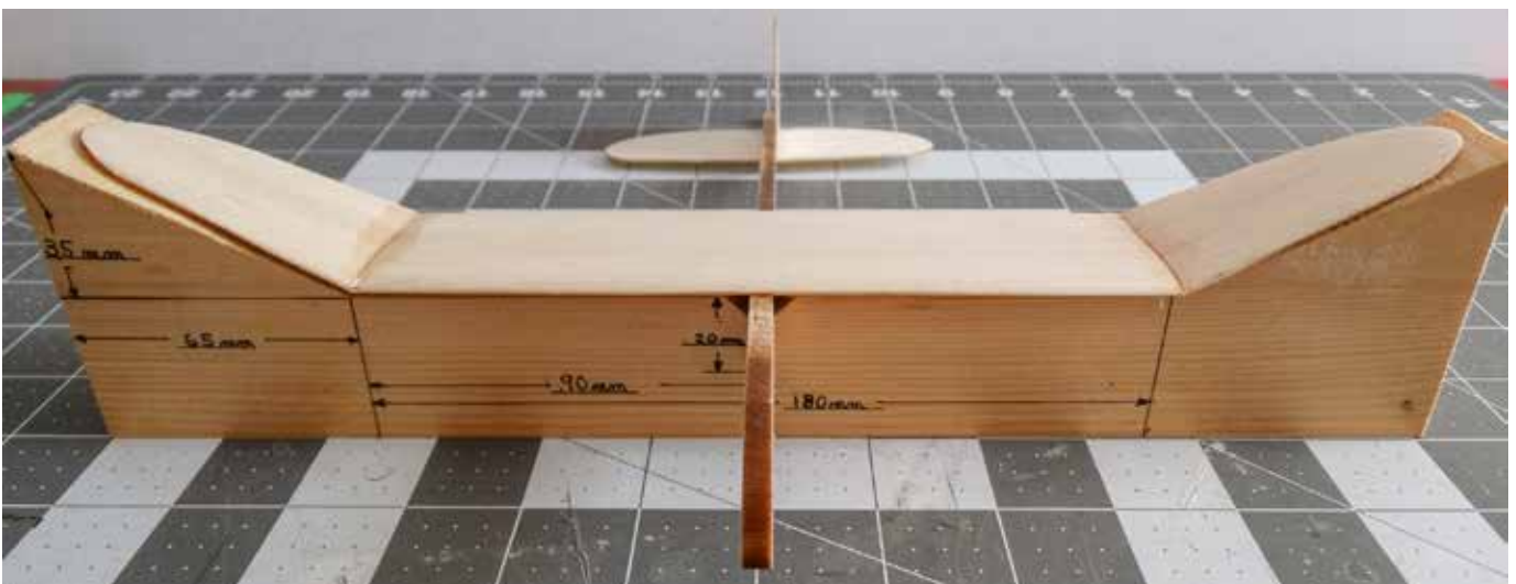
A handy wing jig if you are building several Sparrows in group projects.
