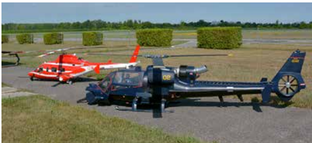
Donovan Dow's turbine helicopters. The 1:5.8 scale, 17kg Bell 430 'Japan' in the background and the 1/4 scale, 25kg Blue Thunder in the foreground were on display
