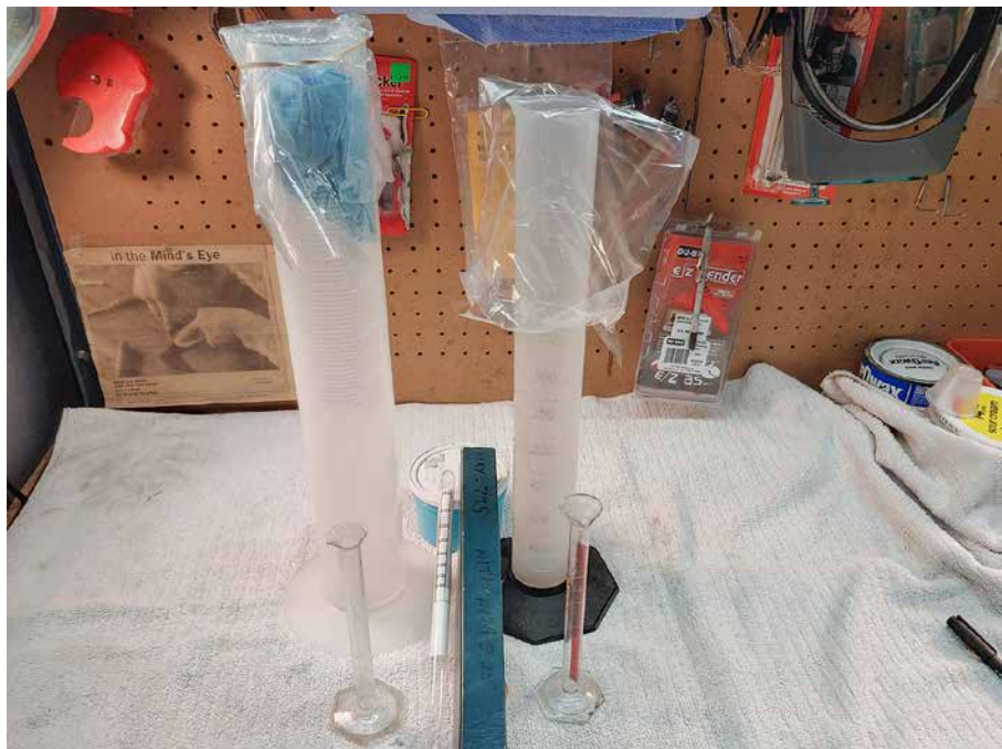
Here are chemistry graduated cylinders of various sizes that I use and a Nurnberg's Hydrometer (for methanol purity testing) / Voici une collection de types acceptables de contenants à carburant.
