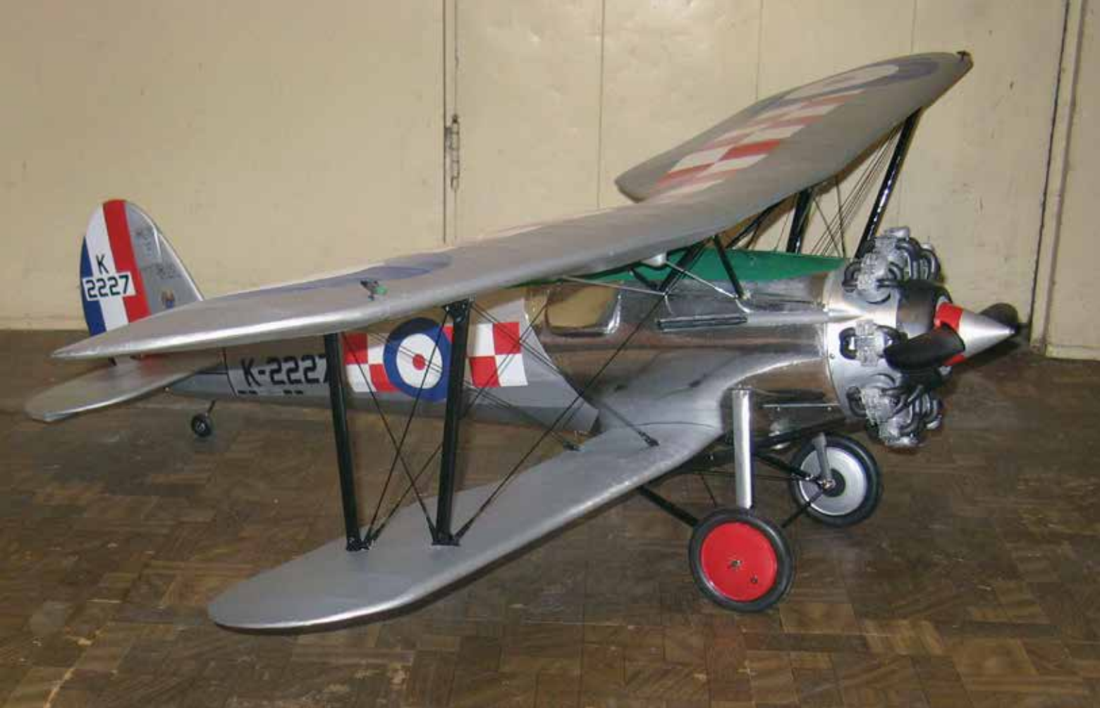
My Bristol Bulldog from Dennis Bryant plans modified for electric power. There are still some scale details to be added.
