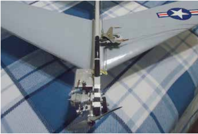
Fury top view showing three-line bell crank throttle control and LA .15 motor.
