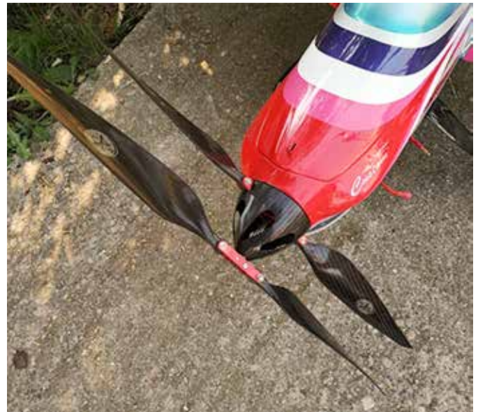
Adam's Twin Motor Contra also sported folding props.
