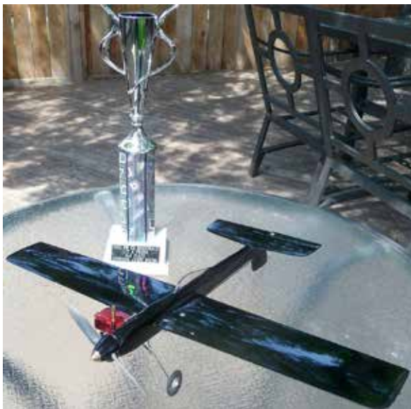
The completed model with all modifications. Placed 3rd first time out at 91 MPH in 2011. Further tuning has upped its current speed record of 97.3 MPH. *Note: Only 1 elevator is needed for control in this event.
