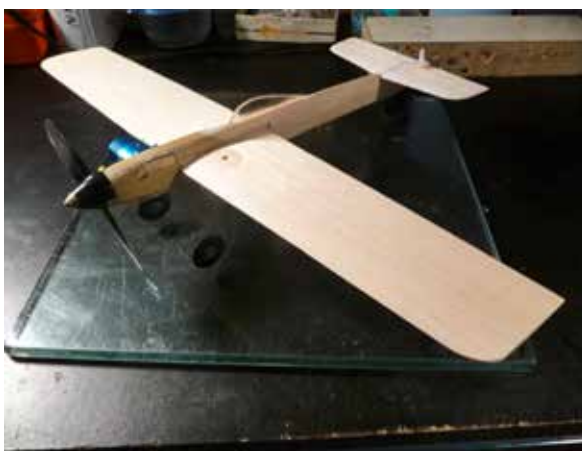
Nearly complete, showing the modifications: Upper fuselage is cut down & rudder removed, stab area reduced, wing area reduced and lightweight landing gear is installed.
