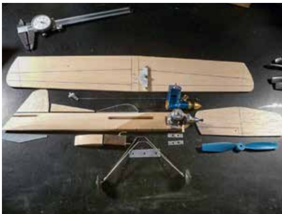
The pre-fab kit parts layout with both original Cox TeeDee .049 engine next to the upgraded Glen Lee Shuriken .05 and Kirn Kraft custom left hand fiberglass prop. *Note:* Only 8 wood parts makes for very easy construction!
