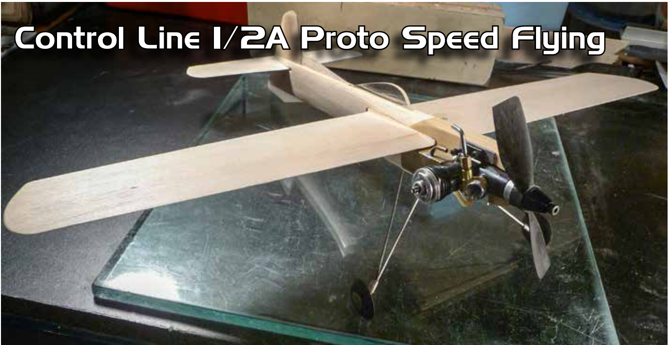
The initial mock up of the stock "TORKY" kit with original Cox TeeDee .049 engine fitted with Left hand crankshaft, homemade L/H carbon prop and metal unflow suction tank. *Note: Wing center section is left square for strongest wing joint fit into fuselage.
