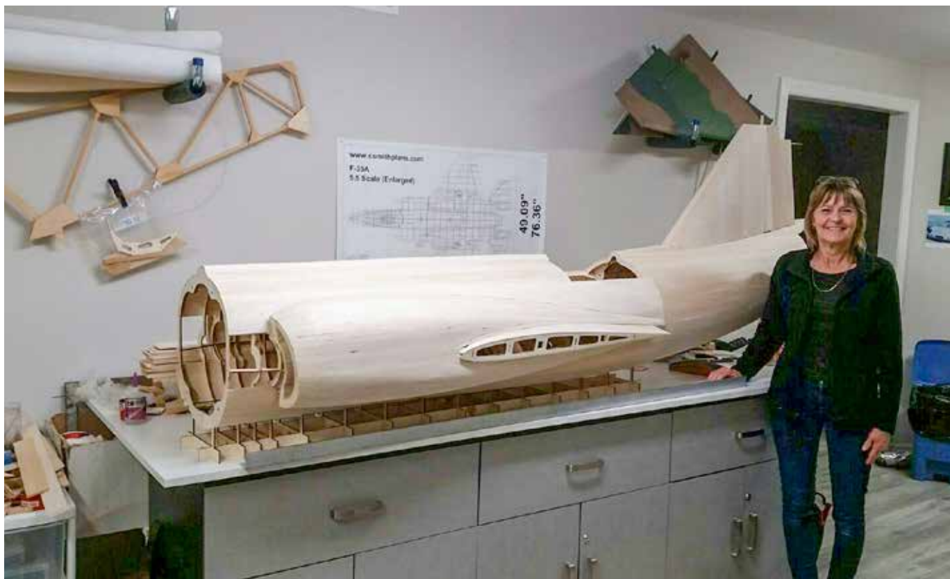
Lynn with Brad Metcalf's quarter scale F-104 jet, in the bones, over 4.2 meters long with a projected weight under 70 pounds. Zoom zoom.
