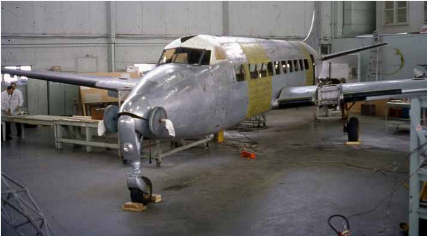
Saunders Aircraft ST-27 under conversion, note the fuselage extensions in green primer.
