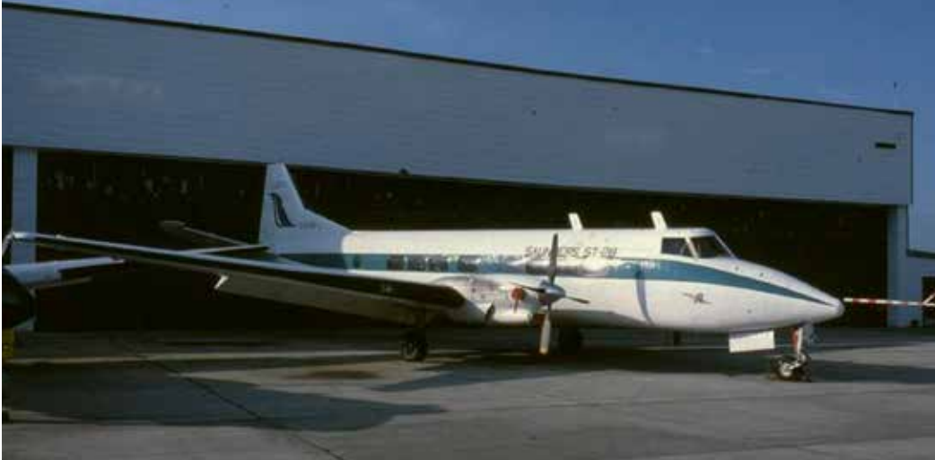
Saunders Aircraft ST-27 under conversion, note the fuselage extensions in green primer.
