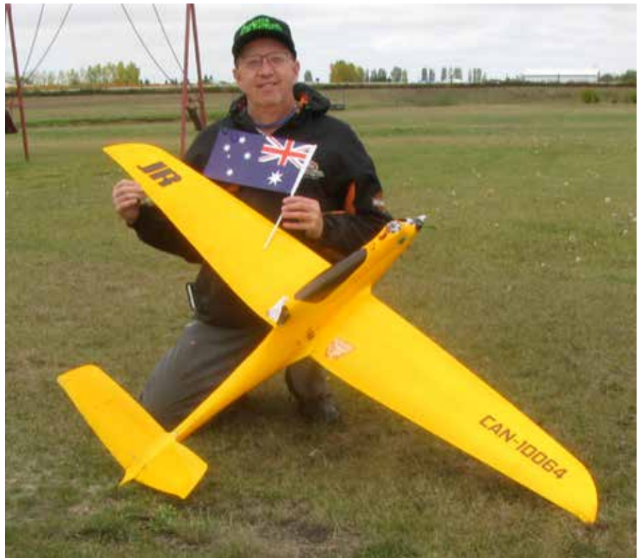
Roy Andrassy with his F3D Pylon plane, Redonkulous, manufactured by Adam Argus in Australia. Engine is MB from Holland with a full wave Paolo Pampana pipe. The propeller is a fully moulded carbon prop from Adam Argus, Radio is JR/DFA with a 28X transmitter. On board glow from Sweden.
