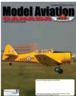
Lee Kelm's 101" Harvard does a fly by at the Chinook Winds field. This beauty is scratch built from Zirol plans, has a Zenoa G62 engine turning a Menz 20 X 10 prop, Robart retracts, and a custom lighting system. Finish is 3/4 oz. glass cloth with epoxy resin and paint is water based enamel.
