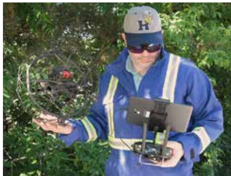
Danny Karaiskakis (#82924) preflights $80,000 Industrial Skyworks specialty Flyability ELIOS copter for an underground drainage inspection (d-labs.ca).
