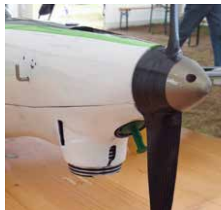
World Championship model used a cool air intake that directs cool air directly to the header.
