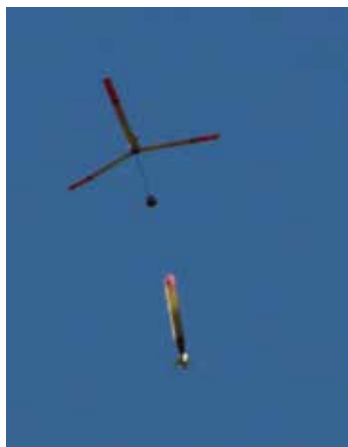
A S9A gyrocopter after it has been ejected but attached to the carrier model. The three blades turn rapidly at 2+ rotations per second. Each blade typically consists of two hinged half span sections which unfurl in flight.
