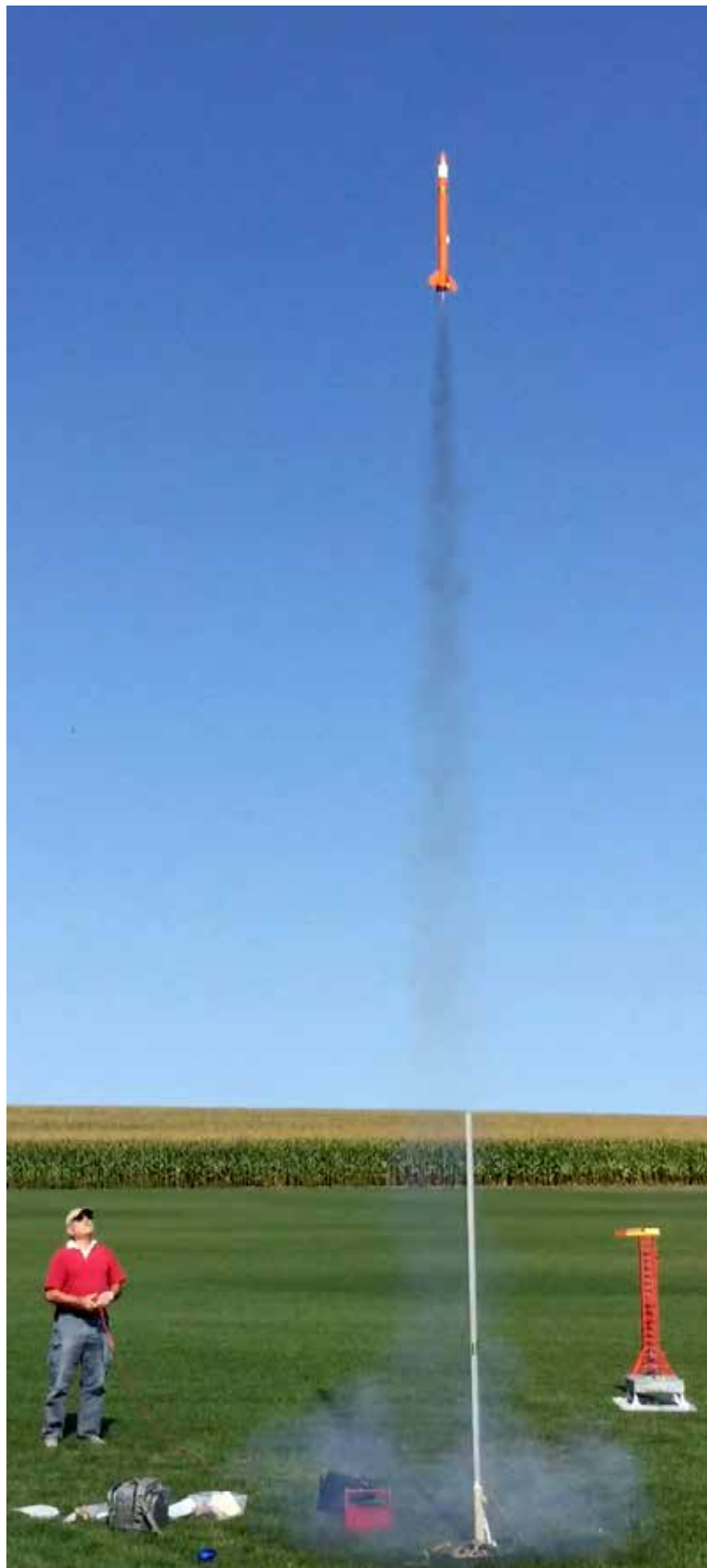
Blast-off of Taras Tataryn's S2/P model during a pre-contest test flight. A long launch rod ensures a straight and vertical boost.
