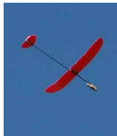
Saverio's S4A model in glide mode with its wing deployed from its folded boost position. This model has a wingspan of about 600 mm. The bulge at the nose of the model is the rocket engine pod. Models weigh less than 30 grams in glide trim.
