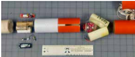
The disassembled payload section of Taras' S2/P model. The components from left to right are: nose cone, altimeters (up to three) and storage compartments, egg "astronaut" and foam protection sleeves, base of payload compartment. The elastic cord keeps the payload and carrier model sections attached during parachute descent.
