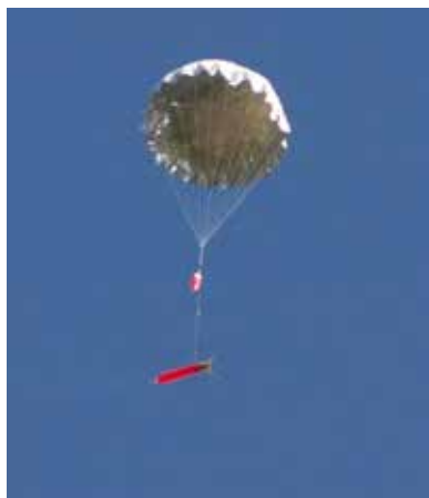
A successfully deployed S3A 1 metre diameter parachute. A large number of shroud lines are used to form the parachute canopy into a high drag sphere. The carrier model is suspended horizontally to create even more descent drag. The aluminized mylar reflects the sun to aid spotting the model in flight.
