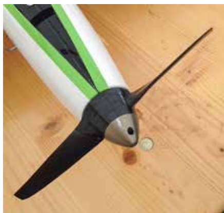
F3D full carbon high performance propellor with moulded hub and titanium spinner nut.
