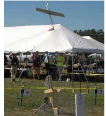
Liftoff of Kevin McLeod's S8E/P model. The contest rules grant only limited radio control of the boost trajectory - just enough to keep it relatively vertical. Too shallow a trajectory and you are disqualified! A 40 N-s "E" class engine will boost the model to 200 metres in altitude.
