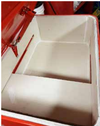
This is a charging station that was built out of an old unused parts washers for automotive parts. It's been lined with gyproc to try and keep an failed lipos contained.
