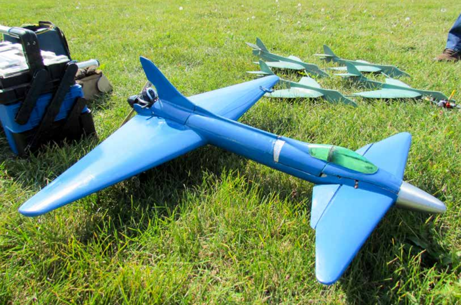
Jack Nagao's Control Line canard, powered of O.S. LA. 15, 2.4 Ghz radio for throttle control.
