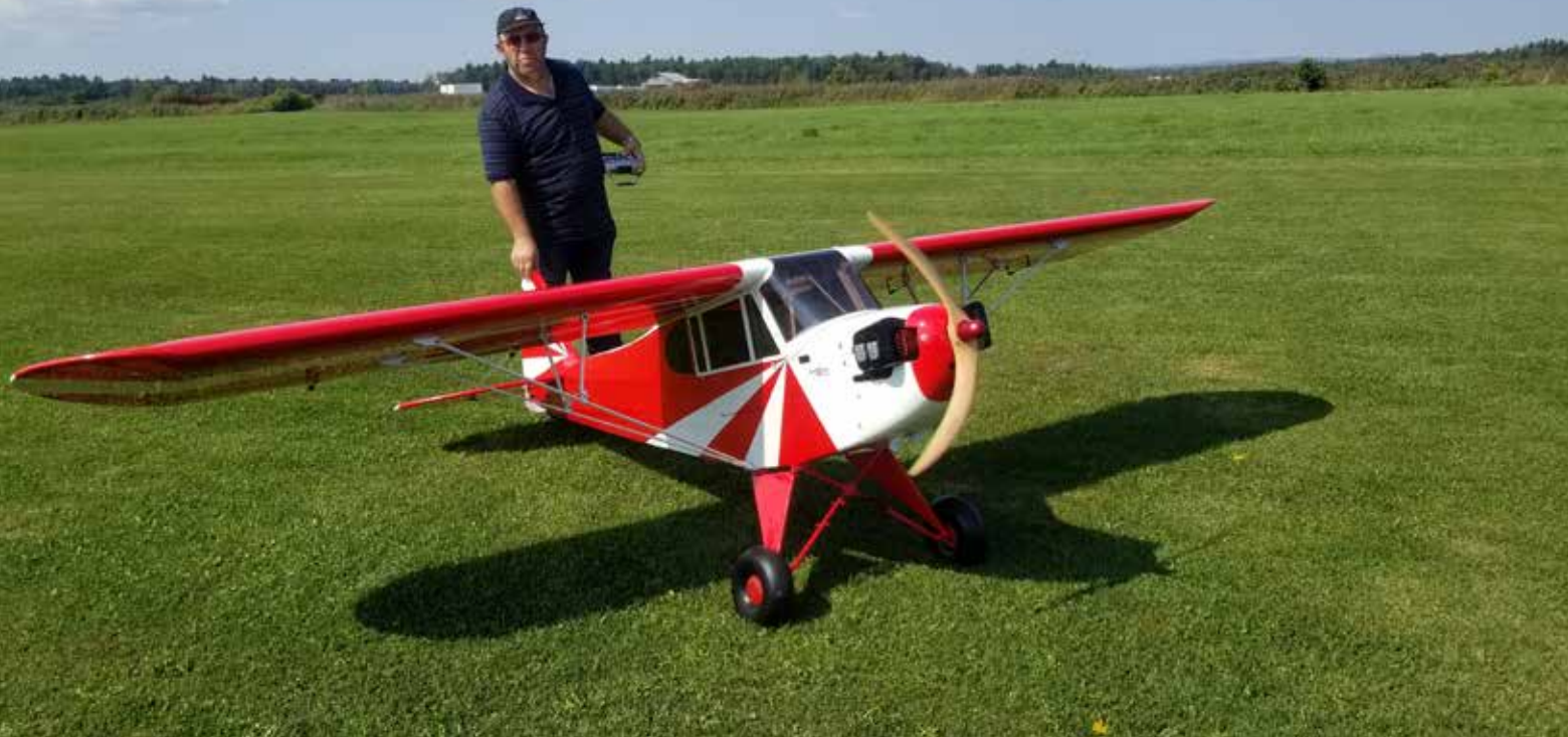
Above: David Janashvili with his incredibly beautiful and realistic 140 inch wingspan 40% clipped wing cub . It is powered by a 3w 106 cc twin cylinder engine!
