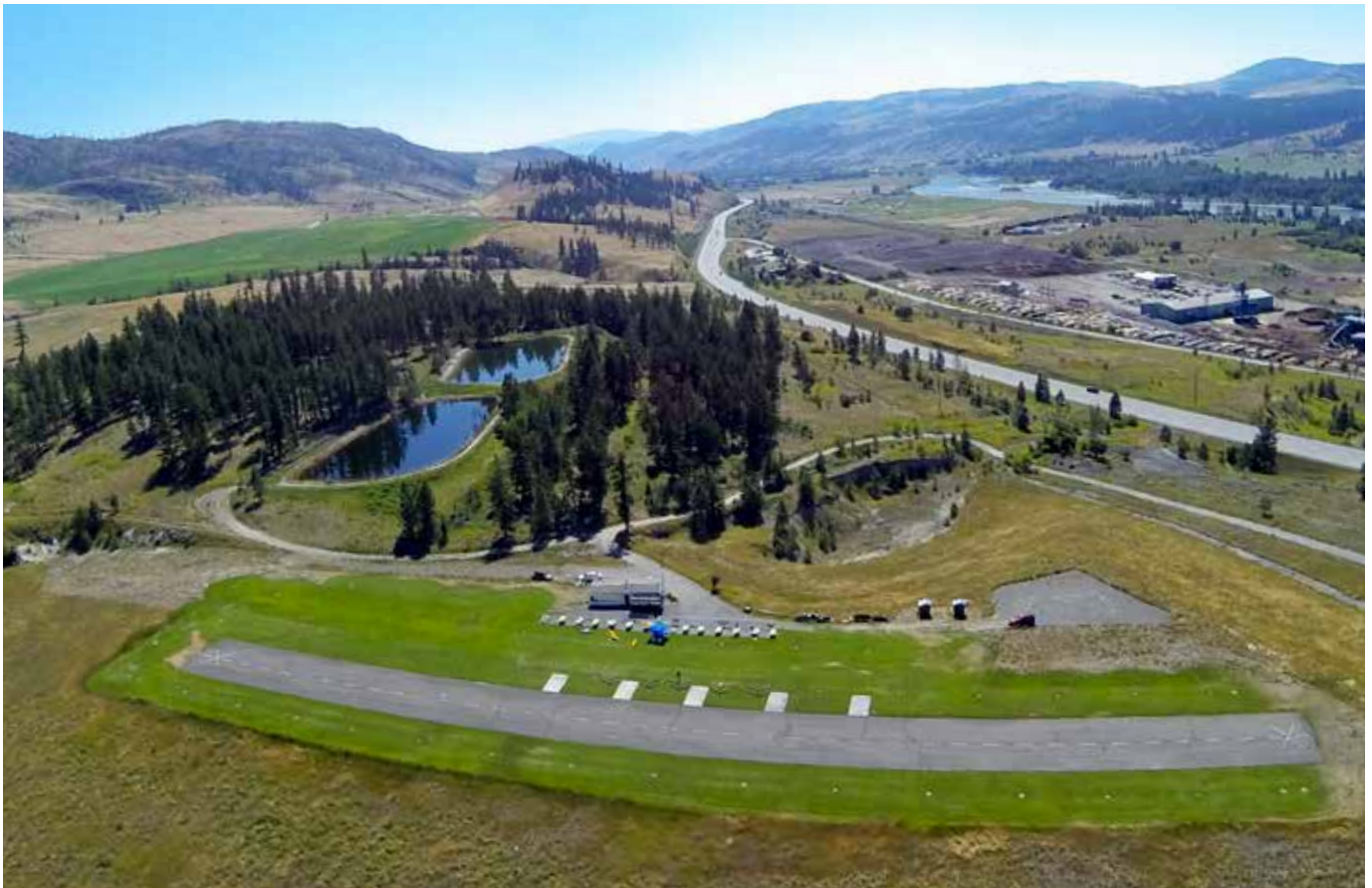
Kamloops Model Airplane Society from the air. KMAS has a 600' x 40' paved runway, electric power on-site, underground sprinklers, a clubhouse, remote weather station and irrigation supply ponds.
