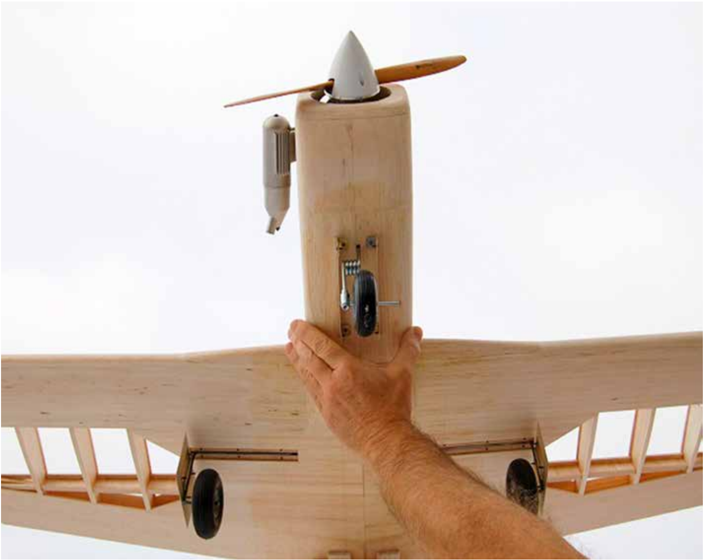
Above: The under carriage of the Mooney/Mark 21 Semi Scale model after the landing gear is installed.
