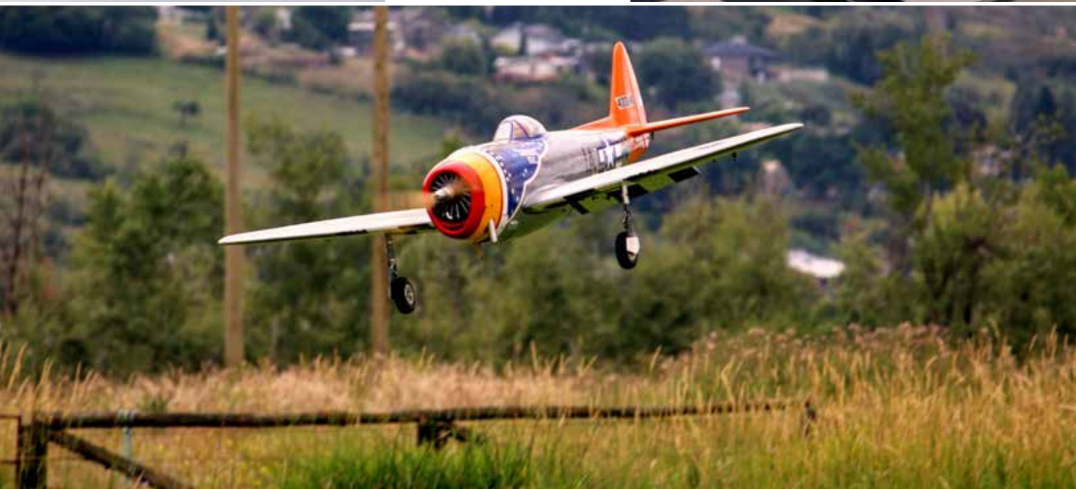
Opposite bottom: Keith Bennett's 74", 8lb, 1/4 scale Balsa USA Sopwith Pup cuts through the skies using a 170R3 Saito radial engine.
