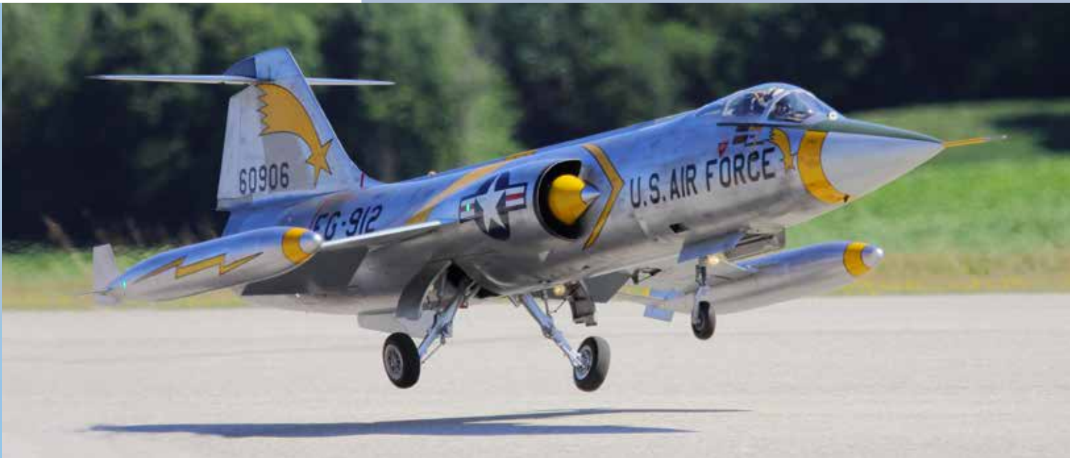
Ali Machinchy's 1/4 scale Airworld F104 Starfighter, with a Jetcat P300 turbine, flares as it is about to touch down.
