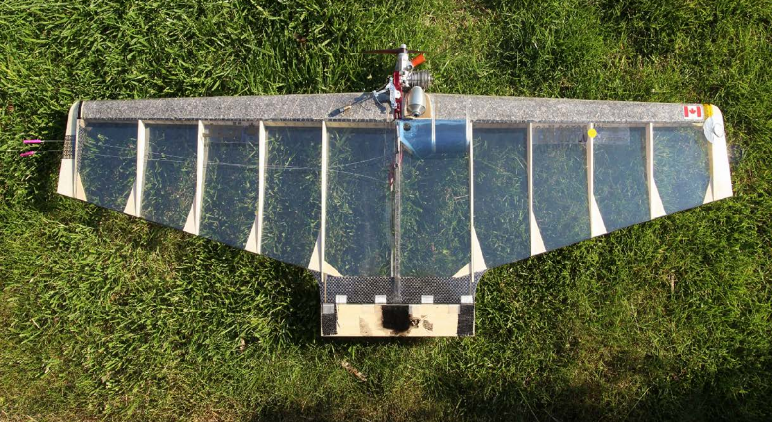
The Team Canada home designed Control Line Combat model, the Jedi, in the straight trailing edge version.
