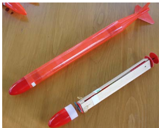
Peter Cook's S9A fibreglass carrier rocket (with gyrocopter loaded) and spare gyrocopter.
