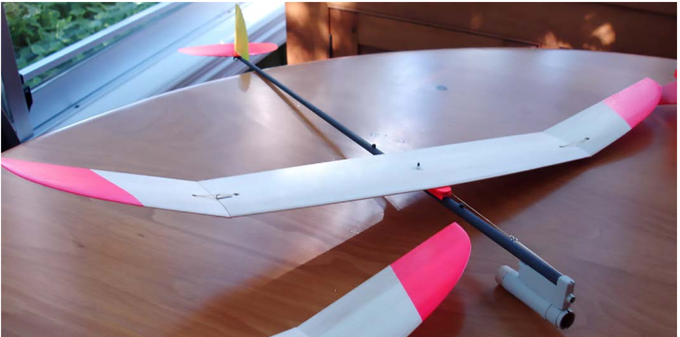
One of Peter Cook's S4A scissor wing models shown in glide configuration. The model wing span is 600 mm. The wing tips fold in and the wing rotates to rest along the carbon fibre fuselage for minimal drag during rocket assisted launch.
