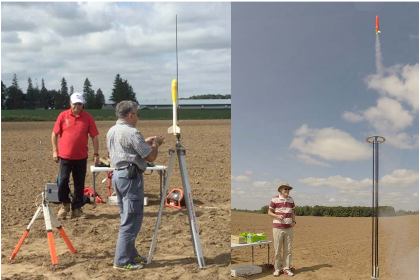
Taras Tataryn (foreground) and Saverio Prato preparing Taras' S2/P model for a pre-contest test flight. The egg "astronaut" is flown in the top payload section. The model is recovered by parachute. An onboard altimeter records flight data. / Pre-contest test launch of Peter Cook's S6A model.
