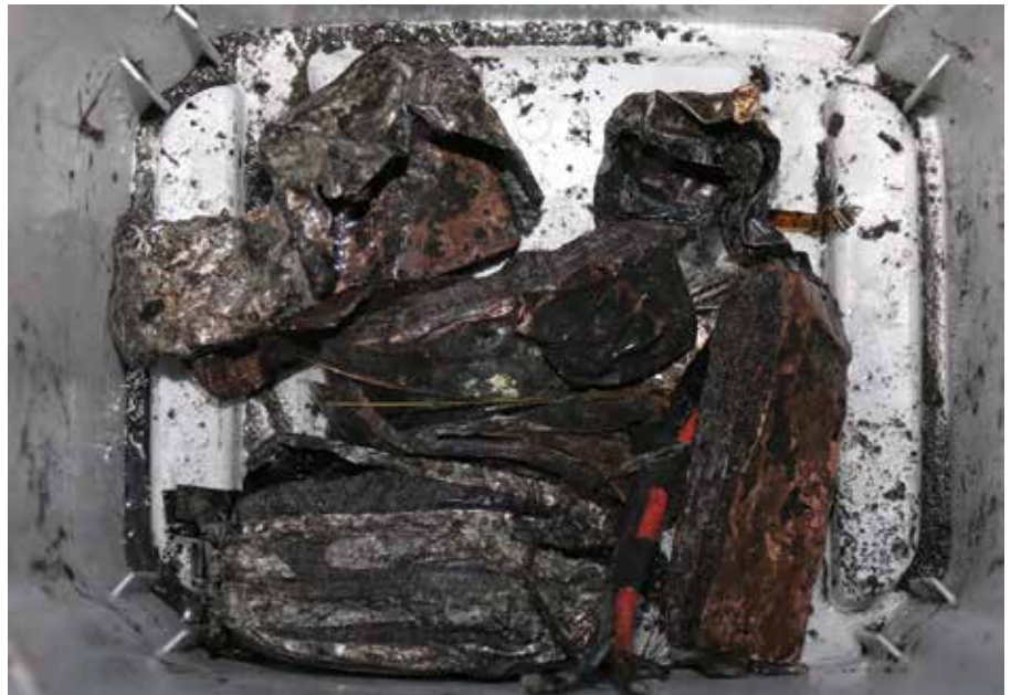
Above: All that is left of the 6 cell LiPo battery from my Edge 540T crash.
