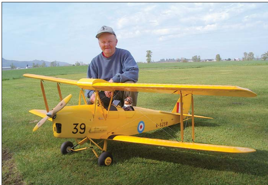
Abbotsford Hawks member Bill Pottage's 1/4 scale Tiger Moth 82a. This beautiful airplane is covered in Solartex and is powered by a Ryobi 30cc engine. It was scratch-built from Clarke Industry plans, and features a 20X6 Clarke scale propeller. It has an 88" wingspan, 2200 sq. in. and weighs in at 21 pounds. Picture was taken by the late Tom Hammond. / Le Tiger Moth 82a de Bill Pottage (un membre des Abbotsford Hawks). Cette maquette splendide est recouverte de Solartex et est mue par un Ryobi de 30 c.c. Bill l'a construit de façon artisanale grâce à des plans de Clark Industry. Une hélice Clarke de 20 X 6 fournit la traction. L'avion possède une envergure de 88 pouces et elle pèse 21 livres. Le regretté Tom Hammond a pris la photo.
