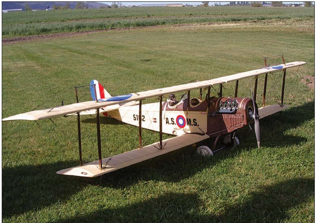
Abbotsford Hawks member Lea Sheppard's beautiful Curtiss "Jenny" JN4 with an approximately 87-inch wingspan and coming in at approximately 14 lbs. This model is powered by a Saito .82 four-stroke. Photo by Tom Hammond. / Le Curtiss Jenny JN4 de Lea Sheppard (un autre membre des Abbotsford Hawks). Envergure d'environ 87 pouces et poids d'approximativement 14 livres. Motorisation par un quatre-temps Saito .82. Une autre photo du regretté Tom Hammond.
