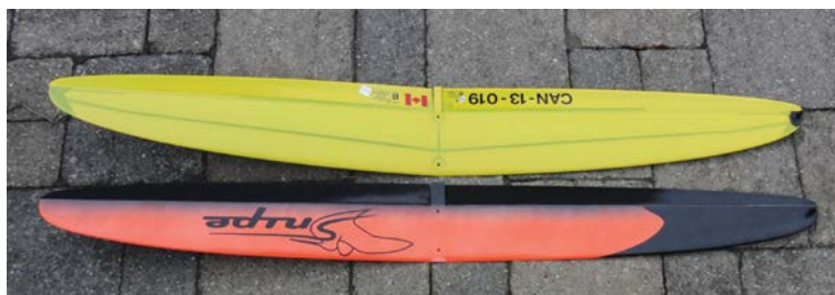
Standard AR Blaster 3 Wing vs. High AR Snipe Wing
