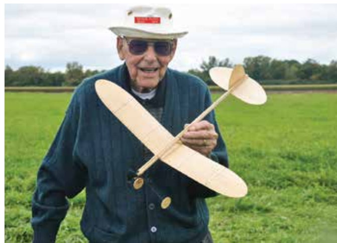
George Parry holds his Cloud Tramp. This simple design is easy to build and flies extremely well. It is a far cry from the drug store models many tried in their youth. Photo by Richard Barlow
