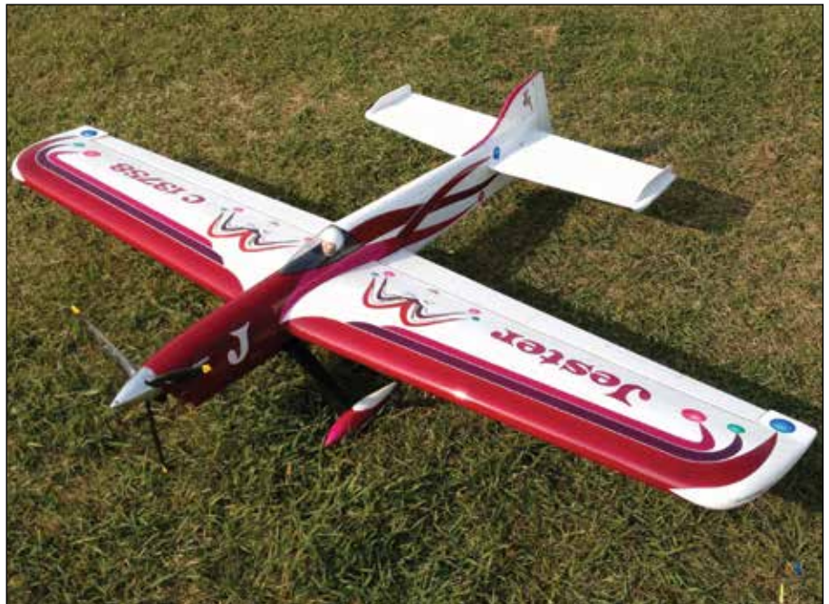
Bruce Perry's Jester with stabilizer tip plates. / Le Jester de Bruce Perry muni de plaques stabilisatrices.
