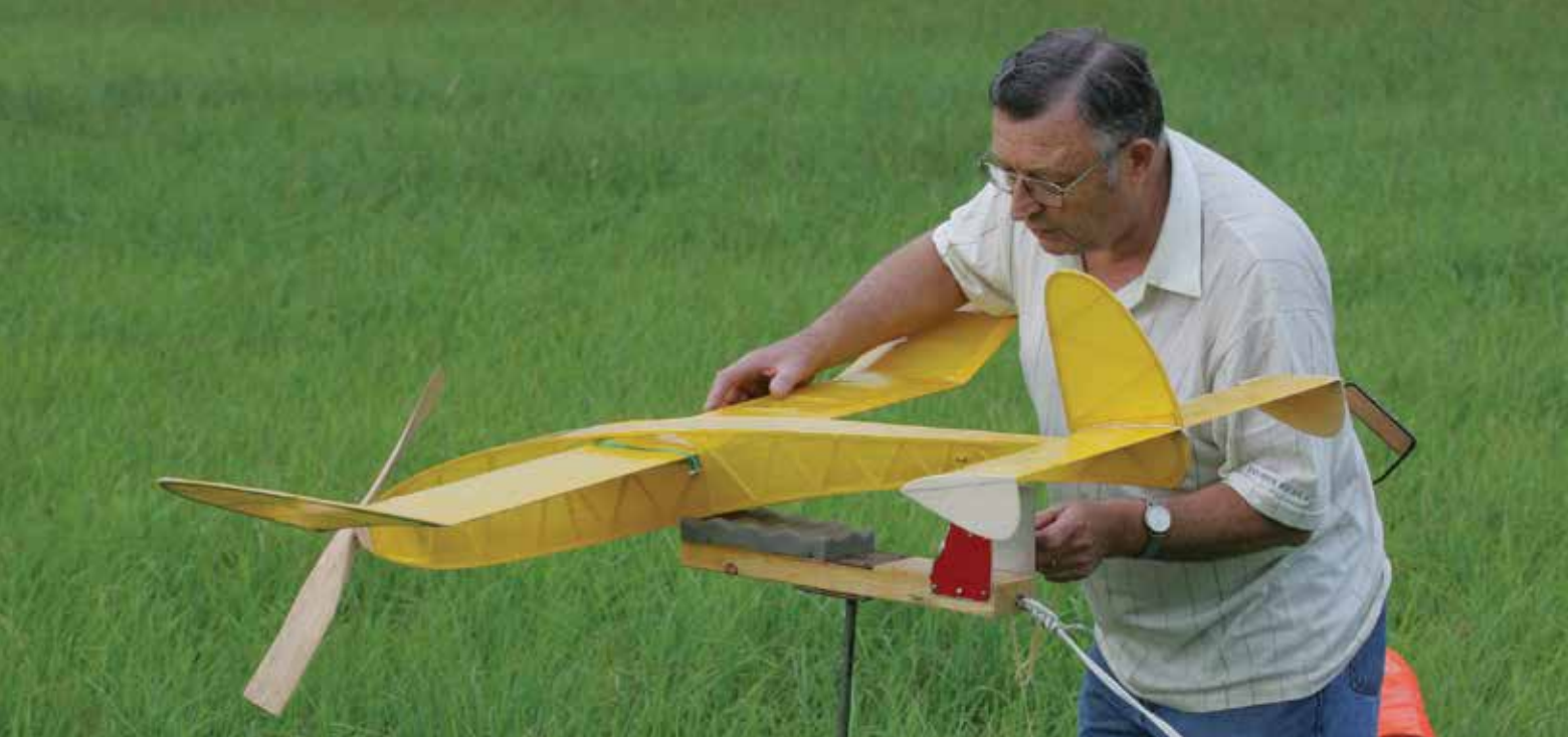
Dave Lonergan prepares his 59" Banana Fritter for flight. Power is from 20 strands of 1/4" rubber flying weight of 426 grams. Photo by Craig Limber.
