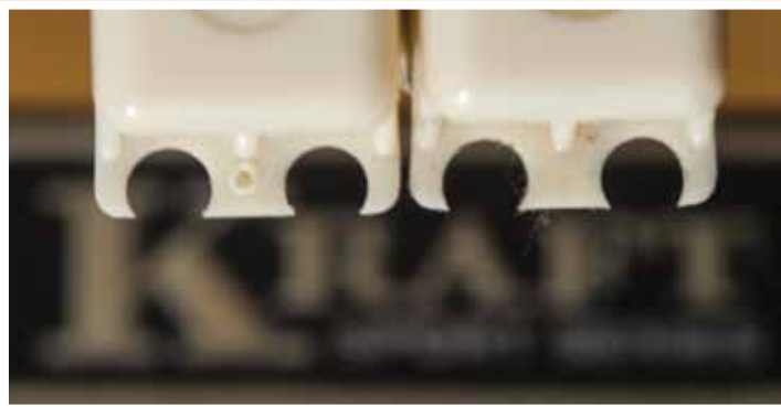
Servo reversing wasn't common on radios until the 1980s, previously modelers would have to identify the rotation of the servos by looking for a mark on the mounting flange. Needless to say, radio installation took more planning without transmitter side servo reversing and end-point adjustment.
