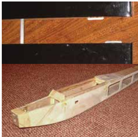
Close-up of construction details of the fuselage, and the tabs added to prevent wing rotation
