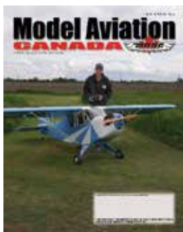
Geoff Dryers poses with his electric powered 50% Clipped Wing Cub in the Hazel Sig colours. The model is scratch built, 180 inch span, and is powered by a Hacker A100-10 motor, 4x 6S 6000 mAh batteries (12S2P) Xoar 27x12 propeller, 7500 input Watts
