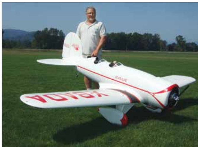
Nigel Tarvin poses with his scratch built Lockheed Sirius "ANAHUAK." The model has a 126 inch wingspan, weighs 42 pounds and is powered by a Zenoah GT-74 twin cylinder engine. Nigel built this model from his own plans and flies it very well. / Nigel Tarvin exhibe son Lockheed Sirius ANAHUAK de construction artisanale. Envergure de 126 pouces, poids de 42 livres et mû par un Zenoah GT-74 bicylindre. Nigel a construit cette maquette depuis ses propres plans et elle vole très bien.
