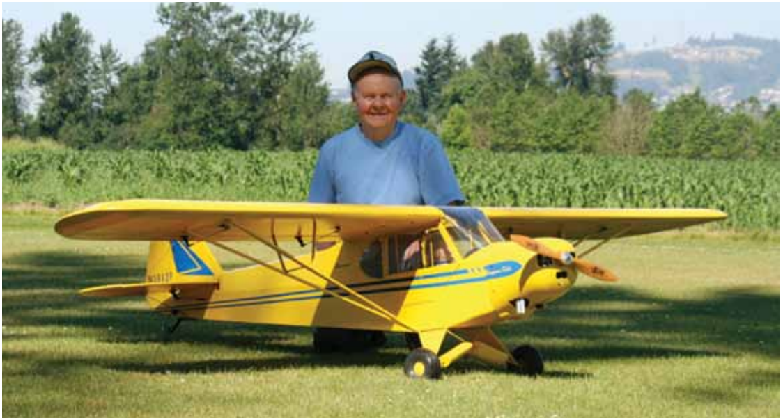
Bill Potage with his 30% giant scale Super Cub, from Wendell Hostetler Plans, 127-inch wingspan, powered by a Quadra 52 with a 22X8 prop. It weighs in at 25 lbs and is covered in 21st Century fabric. / Bill Potage et son Super Cub à l'échelle 30 %, d'après une liasse de plans de Wendell Hostetler. Envergure : 127 pouces, moteur Quadra 52 et hélice 22 X 8. Poids de 25 livres, recouvrement de 21st Century. Photo by Tom Hammond
