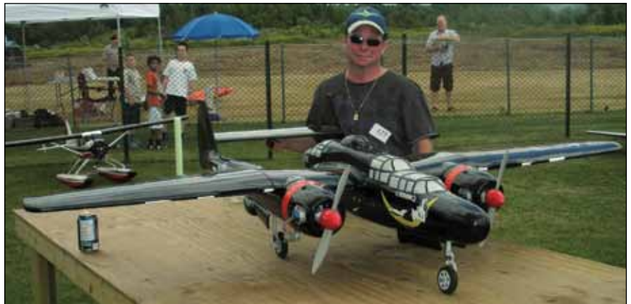
Danny MacLean with his Black Widow P-61 ARF. The model is powered by twin OS.56 four-strokes, spans 79.5" and weighs 12 lbs
