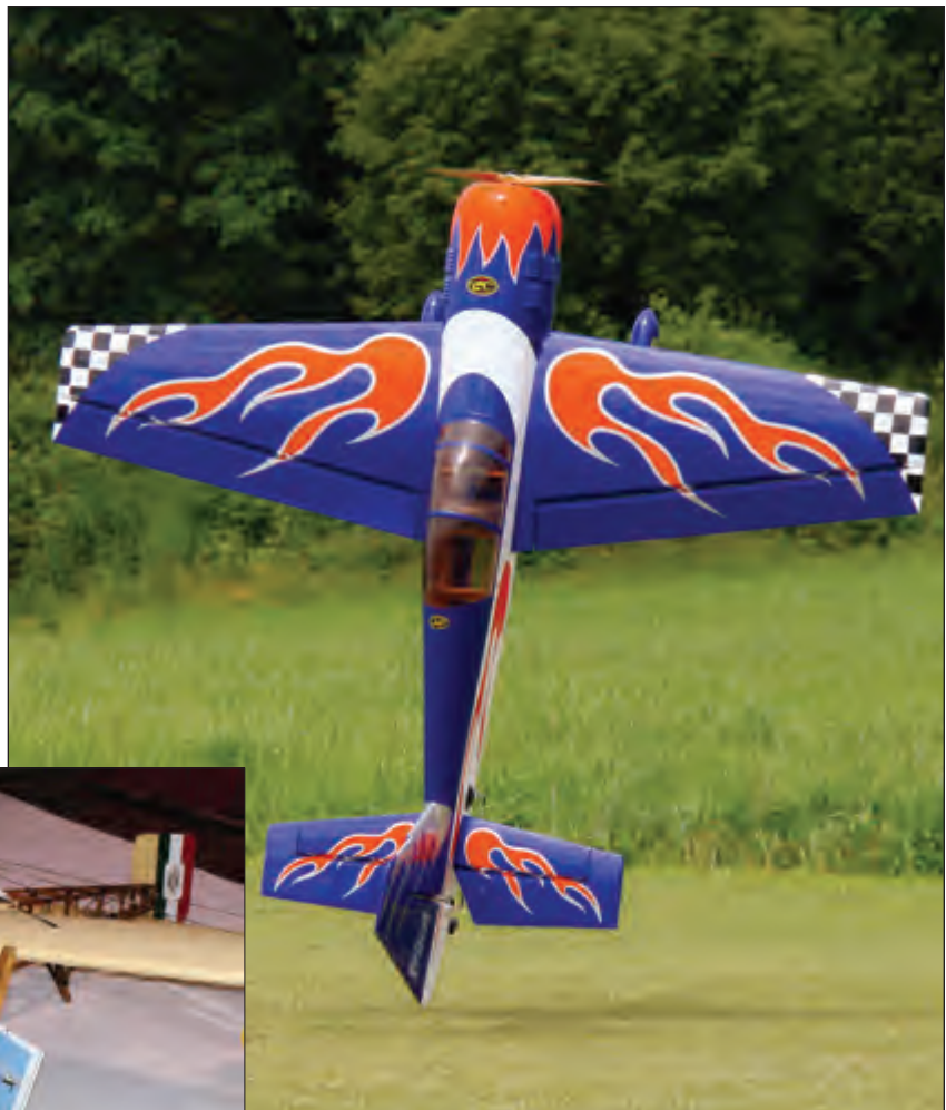
Richard Coyne from Vancouver Island hovers his 88" Yak at the Fraser Valley RC Flyers Field. It weighs 14 pounds, is powered by a Scorpion Outrunner motor, on 10 Lithium polymer cells, swings a 24X12 prop, giving it totally unlimited performance for approximately 8 minutes. Photo by Kevin Sumner
