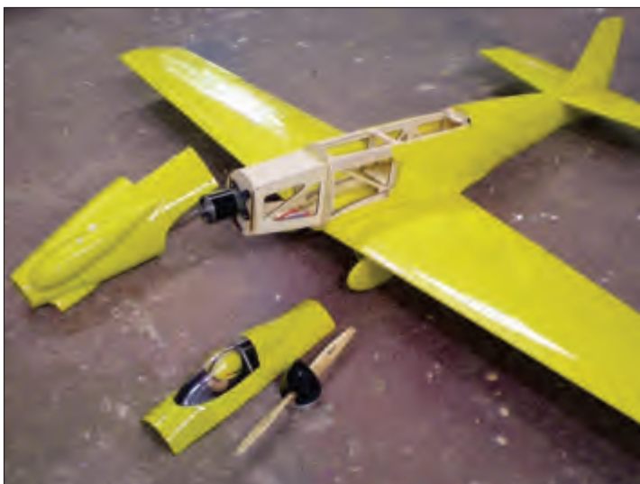
This is the LR-1 designed and built by Jerry Small. You can see the high-quality laser cut ply built-up construction. Some parts like the cowling, canopy and turtle deck are made from molded fiberglass. Most of the airframe is standard built-up construction with shrink plastic covering. / This is the LR-1 designed and built by Jerry Small. You can see the high-quality laser cut ply built-up construction. Some parts like the cowling, canopy and turtle deck are made from molded fiberglass. Most of the airframe is standard built-up construction with shrink plastic covering. / PHOTO: Jerry Small
