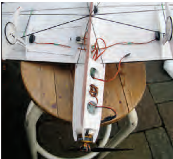
A look at the business side of the model showing the bellcrank and servos. / Les entrailles de la maquette : le bellcrank et les servos.
