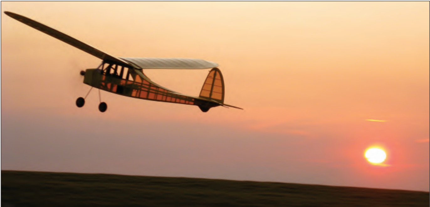
Bill McCormick's Junior Playboy in the air near Tudor, Alberta. The old timer is built from a kit from Barrie, Ontario manufacturer Spirit of Yesteryear. It is powered by a geared Astro Cobalt 05 running on six cells. Photo by Chris Gregg
