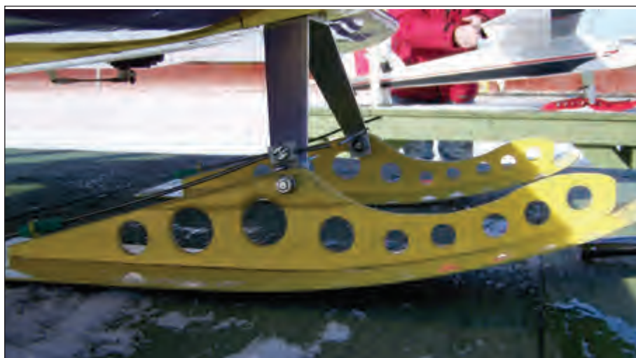
Picture showing the torsion bar set-up on a .40 size Twist that belongs to Jon O'Reilly of the Brockville Model Aeronautics Club. / Photo montrant l'installation (cette fois, de barres de torsion) sur un Twist .40 qui appartient à Jon O'Reilly, du Brockville Model Aeronautics Club.
