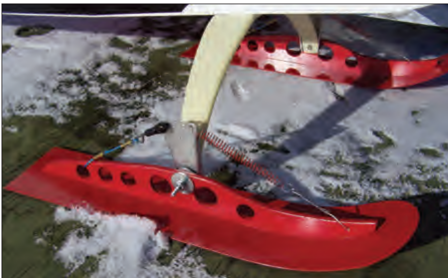
Picture showing the spring and shock cord set-up on a Kadet LT 40 that belongs to Ross Thomson of the Brockville Model Aeronautics Club. / Photo montrant l'installation (ressort et corde élastique) sur un Kadet LT 40 appartenant à Ross Thomson, du Brockville Model Aeronautics Club.
