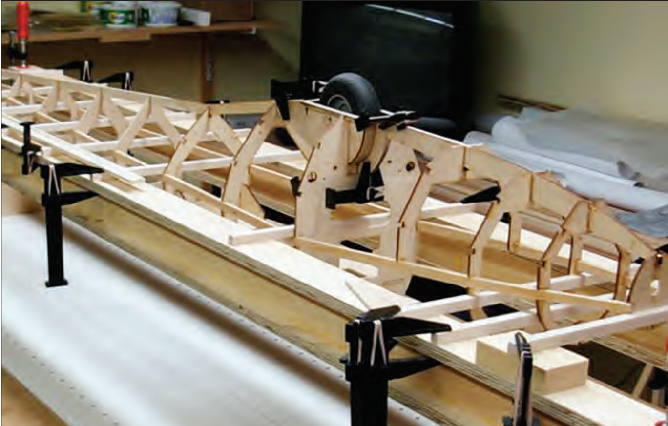
Keith Bonner's ASK-18 under construction. Note his arrangement for aligning the formers of the fuselage! / L'ASK-18 de Keith Bonner en construction. Regardez comment il aligne les formers du fuselage!
