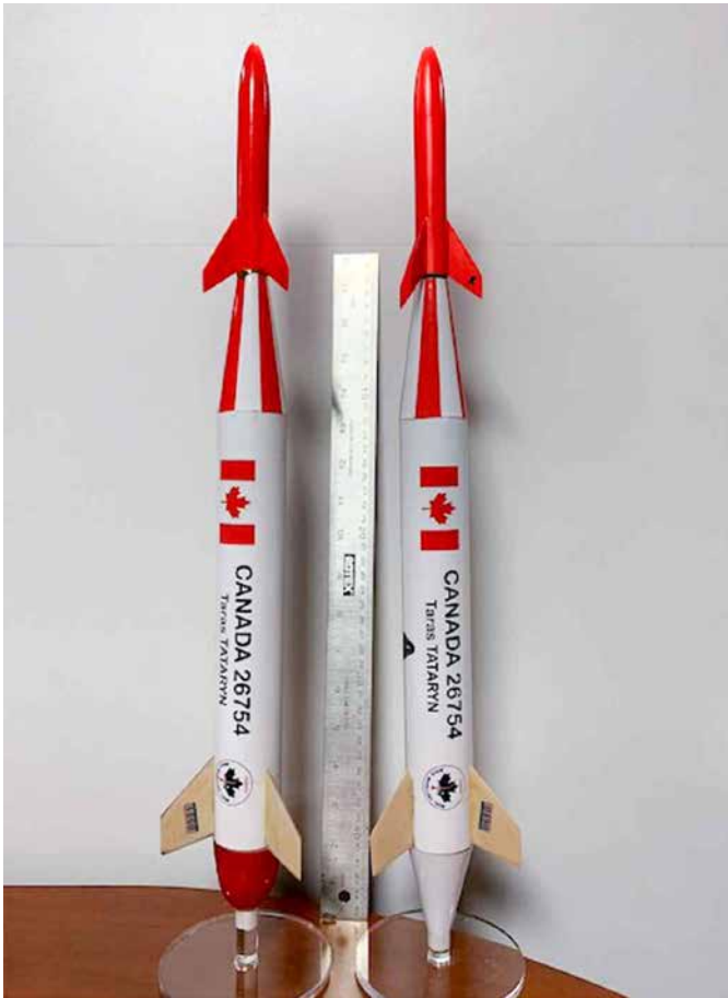
Taras Tataryn's S1B entries. Event rules specify the minimum diameter and length of the cylindrical section of the model. This translates into a large booster section for best altitude performance. The high drag booster only propels the model up about 50 m. The small, low drag upper stage carrying the altimeter then separates and flies on its own. The booster section is a rolled cardstock tube. The upper stage consists of a lightweight fiberglass tube with balsa nose cone. Some boost stability issues could be due to the too far forward placement of the booster fins.
