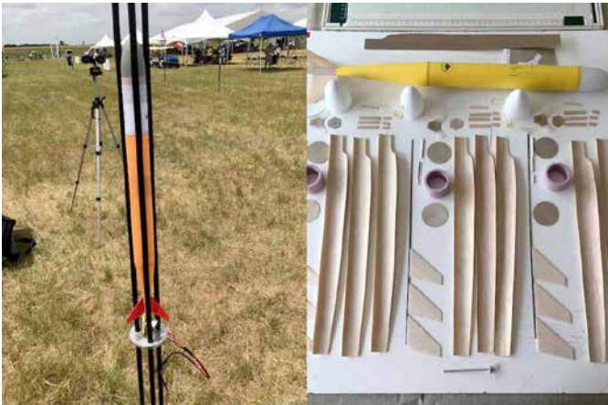
My S9A model ready to launch. The body was formed out of card stock wrapped around a body tube mandrel. A roll pattern was printed on the card stock. The 3 bladed helicopter device is folded up inside the tube for launch. While simpler to manufacture than fiberglass bodies, the extra few grams of weight hurts flight time. The model was launched from a three-rod tower. The use of a piston launched which augments engine thrust is really need to be competitive.
