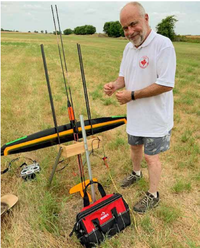
Mike Dennett's S8P model on the Launch Pad. Rails are used to initially guide the model up while it is moving too slow for the control surfaces to be effective.
