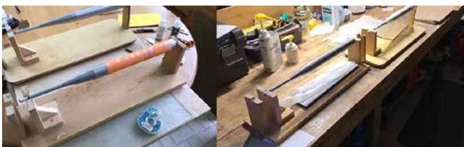
A body tube being formed out of cardstock material. An aluminum mandrel is used to shape the tube. The wrap is taped together until the glue in the seam hardens. This method enables tubes to be quickly manufactured out of inexpensive material. They are a little heavy and obviously not practical to use if launch conditions are damp.
