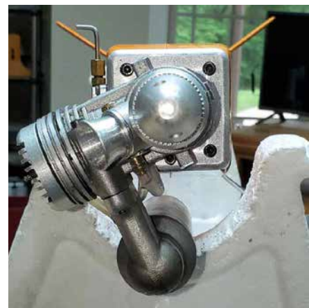
This is a picture of the 25-degree engine rotation mount. Note that the lower left mounting hole is not accessible because the cylinder is in the way. Also note that an additional 6-32 attachment hole is provided for a fourth bolt, if a person wanted to use it.
